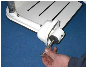
4 – return pivot bolts to pivot assembly once the flanges are unattached
