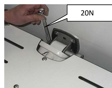
16 – tighten the three pivot bolt and nut to 20N of force. The seat should move up and down with a small amount of user efforts, and should not move independently
