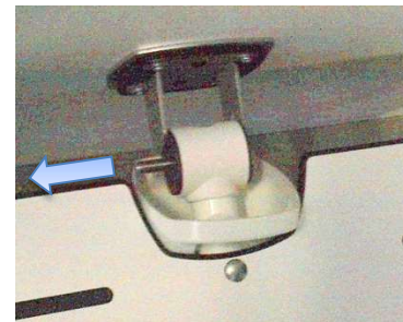
13 – remove the pivot bolt
