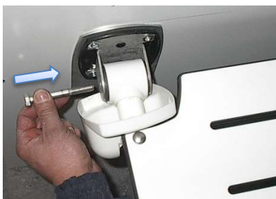
15 – thread pivot bolt through flange plate hole, pivot assembly, and out the other side of the flange plate hole
