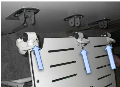
12 – with flange covers pulled back, position the seat pivot assemblies near the flange
