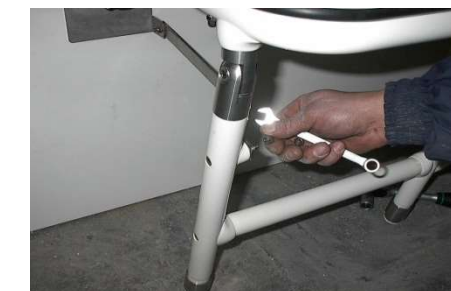
17 – refasten the hinge bracket to each leg
