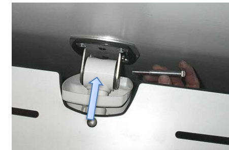
14 – align pivot assemblies with the flange holes.
