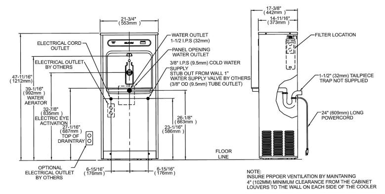
NEW INSTALLATIONS MUST USE GROUND FAULT CIRCUIT INTRUPTER (GFCI) IT IS HIGHLY RECOMMENDED THAT THE CIRCUIT BE DEDICATED AND THE LOAD PROTACTION BE SIZED FOR 20 AMPS
