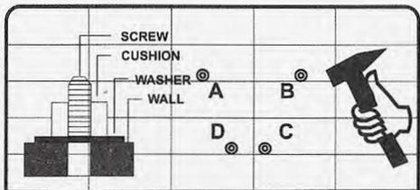
**3** REMOVE THE MOUNTING INSTRUCTION SHEET. HAMMER THE DOWELS SUPPLIED INTO THE FOUR HOLES.
