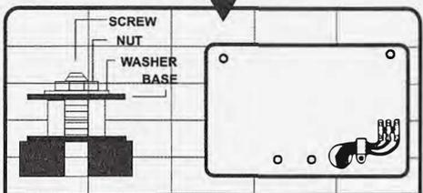
**6** INSTALL THE HOUSING BACK TO THE BASE PLATE BY DECLINING 10 DEGREES AND SECURE THE HOUSING IN PLACE.
