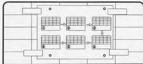
**1** FIX THE MOUNTING INSTRUCTION SHEET TO THE WALL WITH HOLES C AND D 130CM FROM THE GROUND.
