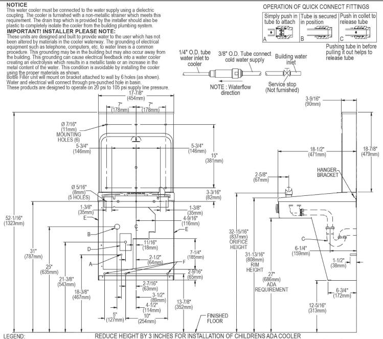
A = Recommended Water Supply location. Shut-off Valve (not furnished) to accept 3/8" O.D. unplated copper tube. Up to 3" (76mm) maximum out from wall.
