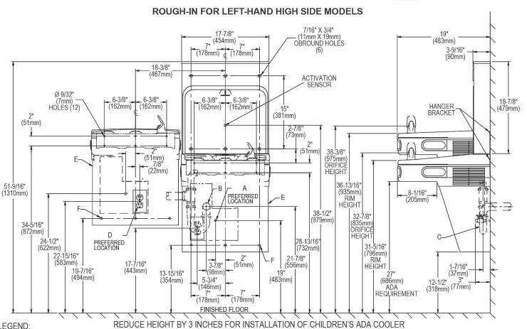
A = Recommended Water Supply location. Shut-off Valve (not furnished) to accept 3/8" O.D. unplated copper tube. Up to 3" (76mm) maximum out from wall.
