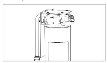
3. Connect a 3/8 inch water supply line, copper or plastic, to the quarter-turn shutoff valve.
