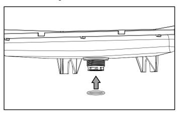
Thread the strainer into the drain adapter.
