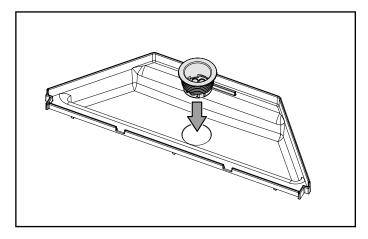
4. Install the O-ring over the strainer threads.
