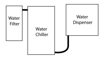
**Note:** The remote chiller can take from 24 to 48 hours to provide completely chilled water.
