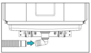
Route the drain hose through the filter box and attach the other end to the p-trap drain adapter using a hose clamp. The drain adapter is designed to be glued into a 1-1/4 inch PVC pipe.
