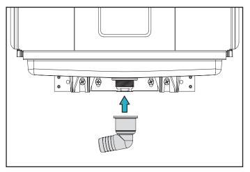
Attach one end of the 3/4 inch flexible drain hose to the 3/4 inch barbed drain adapter connection using the supplied hose clamp. The supplied flexible drain is 13 inches long. If a longer drain hose is required, it must be installer-supplied.
