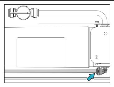
b. If the filter is installed in a remote location, attach an installer supplied length of 1/4 inch tubing to the 1/4 inch tubing from the water dispenser using a union coupling. The type of 1/4 inch tubing, copper or plastic, should meet all local regulations and building codes.
