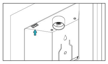
3. Move the power switch to the ON position and make sure the LED lights are lit.
