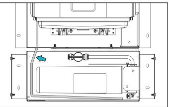
1. Connect the 1/4 inch water line from the water dispenser to the filter housing.
