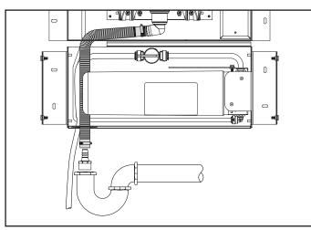
10. Connect the drain adapter into the household waste drain pipe.
