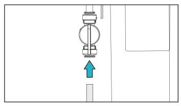
4. Connect a 1/4 inch water line, copper or plastic, to the outlet connector of the filter.
