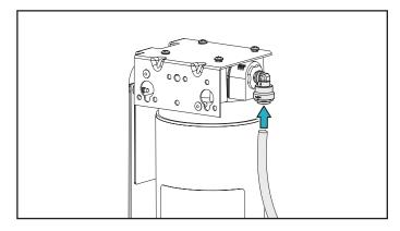
5. Connect the 1/4 inch water line to either a remote chiller or the 1/4 inch water line on the water dispenser. Use a union connection fitting to connect the water line to the water dispenser.
