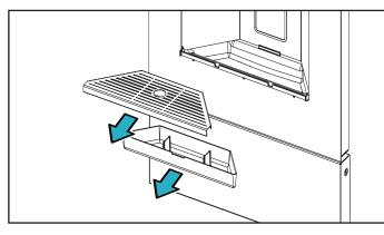
2. Remove the two screws attaching the drain basin to the water dispenser. Remove the drain basin.
