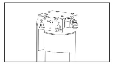
Connect a 3/8 inch water supply line, copper or plastic, to the quarter-turn shutoff valve.
