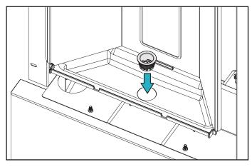
6. Install the O-ring over the strainer threads.
