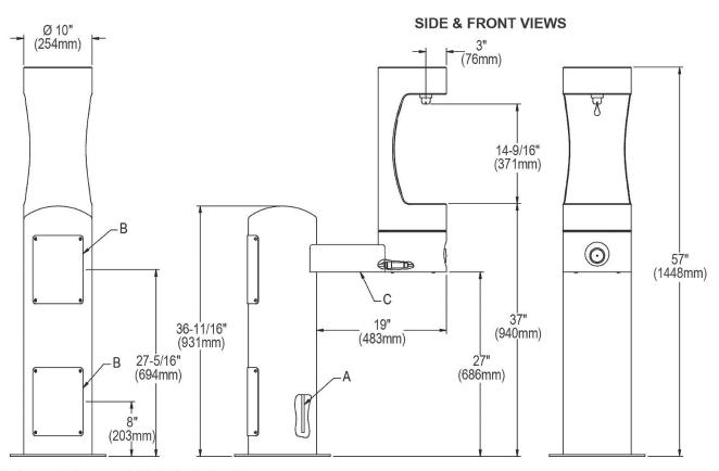
A = 3/8" O.D. Unplated copper tube connect. Shut off valve by others.
