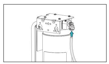
5. Connect the 1/4" insulated water line to either a remote chiller or the 1/4" water line on the bottle filler. Use a union connection fitting to connect the water line to the bottle filler. The type of 1/4" tubing, copper or plastic, should meet all local regulations and building codes. This line should be insulated to prevent condensation.
