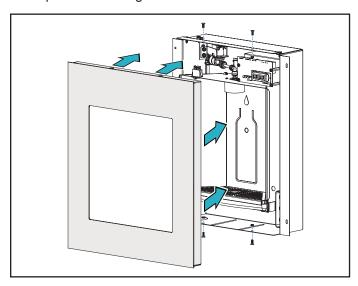
Attach the front cover with the top two mounting screws to prevent it from falling away from the water dispenser while the filter unit is being installed.
