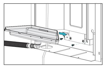
8. If the filter box is used, route the drain hose through the filter box. Attach the other end to the p-trap drain adapter using a hose clamp. The drain adapter is designed to be glued into a 1-1/4" PVC pipe.
