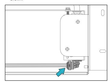
9. Connect an installer supplied 3/8" water supply tube to the quarter-turn shutoff valve, as shown. The type of tubing, copper or plastic, should meet all local regulations and building codes.
