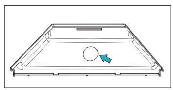
Trial fit the strainer. If the strainer does not fit, carefully open the size of the hole. If it fits well, place a small amount of plumbers putty around the lip of the strainer flange and insert it into the hole.
