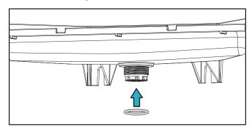
5. Thread the strainer into the drain adapter. Needle-nose pliers can be used to hold the drain adapter from the top while tightening. Ensure that the connection creates a watertight seal. The drain adapter must be facing to the left.
