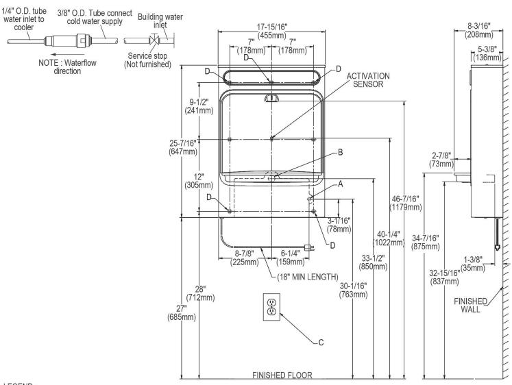
A = Recommended water supply location; 1/2" I.P.S. maximum pipe size. Service stop valve not furnished. B = Recommended location for waste outlet 1-1/4" O.D. maximum pipe size.
