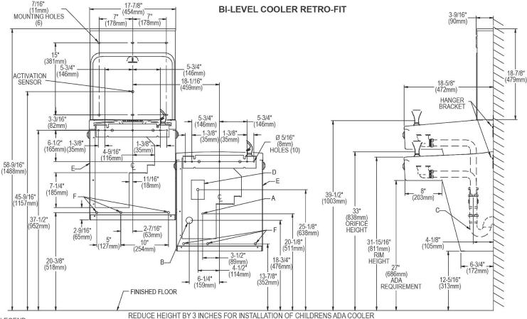
A = Recommended Water Supply location. Shut-off Valve (not furnished) to accept 3/8" O.D. unplated copper tube. Up to 3" (76mm) maximum out from wall. B = Recommended Waste Outlet location. To accommodate 1-1/2" nominal drain. Drain stub 2" (51mm) out from wall. C = 1-1/2" Trap (not furnished).
