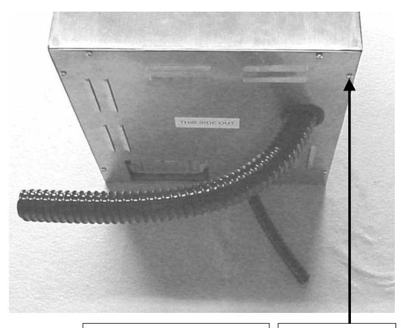
Remove and replace the (2) Plugs with the appropriate Grommets and route the cable or electrical conduit and the factory supplied Drain Hose through their appropriate Grommets prior to fastening the Bottom Plate. Bottom Plate is fastened using (6) AEC1147 screws and (6) AEC1704 lock washers removed at start of installation.
