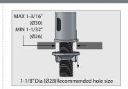
the escutcheon flange (with O-ring down) into the hole in the counter top. Slide the gasket, disk and nut over the black soap tube and both cables and thread onto the shank and secure it to deck underside.
